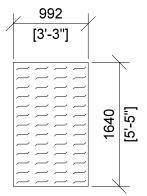
833 Monocrystalline Module 40mm deep with Enphase micro inverters 1 per panel.
